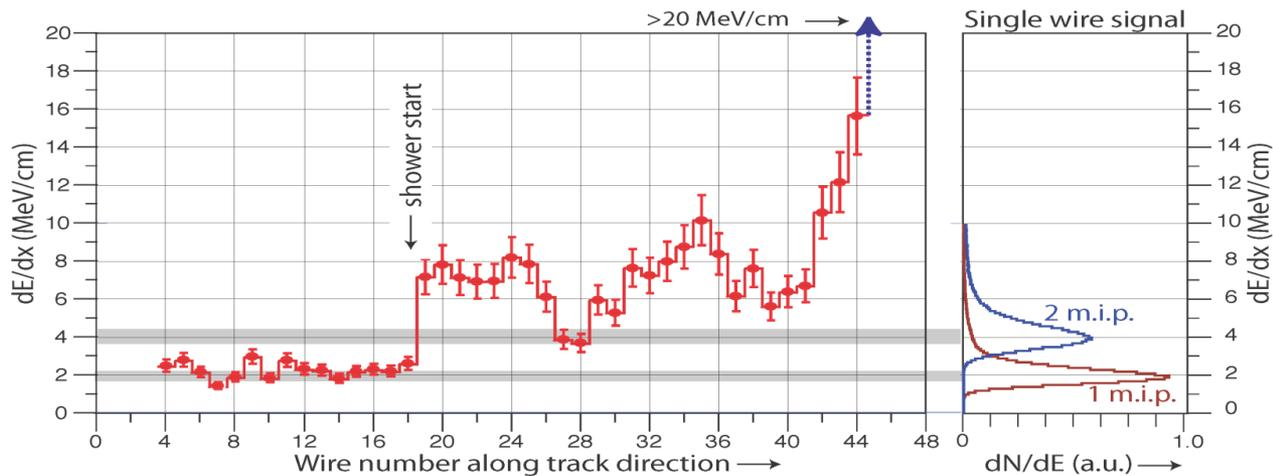
The evolution of the actual  $dE/dx$  from a single track to an e.m. shower for the electron shower is clearly apparent from individual wires.
