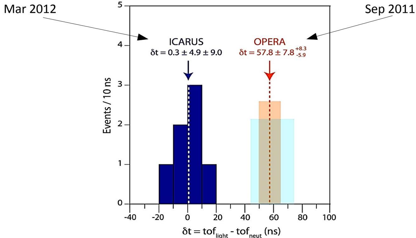
The main measurement error for OPERA experiment concerned the optical fiber connector which was not functioning correctly when the measurements were taken.
